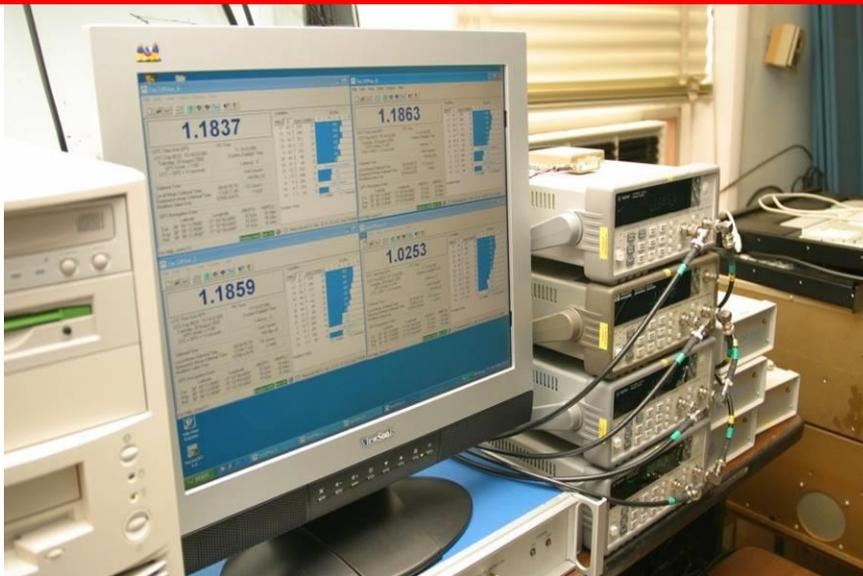
Tac32Plus software simultaneously processes data from four Time Interval Counters and four CNS Clocks, writing 12 logs continuously.
