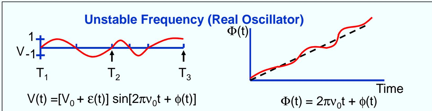
**Instantaneous frequency,  $\nu(t) = \frac{1}{2\pi} \frac{d\Phi(t)}{dt} = \nu_0 + \frac{1}{2\pi} \frac{d\phi(t)}{dt}$**
