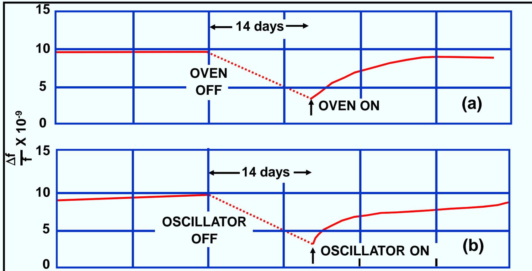
In (a), the oscillator was kept on continuously while the oven was cycled off and on. In (b), the oven was kept on continuously while the oscillator was cycled off and on.
