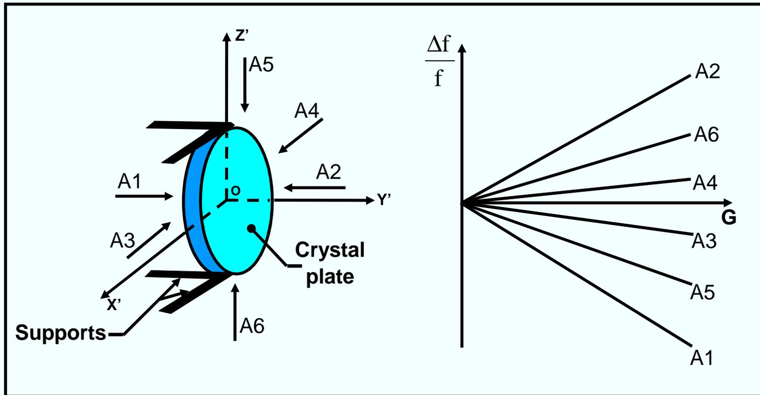
Frequency shift is a function of the magnitude and direction of the acceleration, and is usually linear with magnitude up to at least 50 g's.
