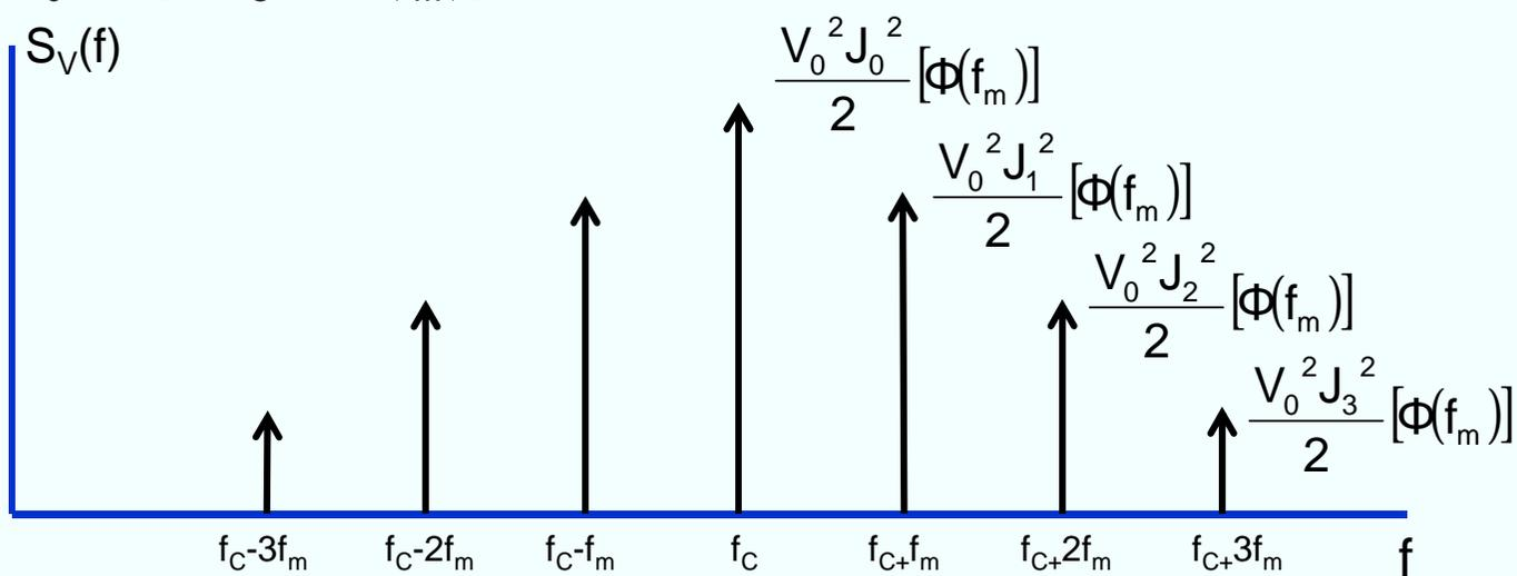
$$\text{SSB Power Ratio} = \frac{V_0^2 J_1^2 [\Phi(f_m)]}{V_0^2 J_0^2 [\Phi(f_m)] + 2 \sum_{i=1}^{\infty} J_i^2 [\Phi(f_m)]} \cong \mathcal{L}(f_m) \cong \frac{S_\phi(f_m)}{2}$$
