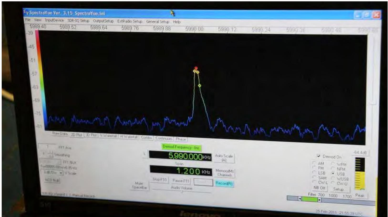
In this case, we see a span of  $\pm 600$  Hz around the Phase Cal “rail”. The Resolution Bandwidth (RBW) is 0.85 Hz and the screen is showing a 40 dB amplitude range.
