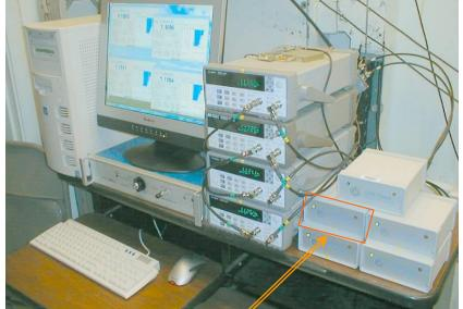
Time Interval Counters compare the 1PPS from each CNS Clock (M12+) against the USNO's UTC time tick.
