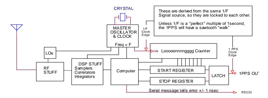
•For the older Oncore, F=9.54 MHz, so the 1/F sawtooth has a range of +/- 52 nsec (104 nsec peak-to-peak)
