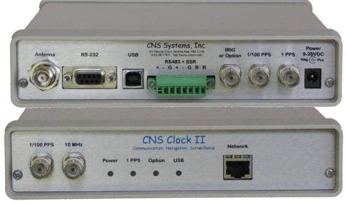
Data available on RS-232, USB 2.0, Ethernet LAN, RS-485 and solid state relay Ports Ethernet NTP Server for your LAN TNC GPS Antenna Connector Buffered 1 PPS outputs GPSDO 10 (or 5) MHz output High Performance PPS Steered TCXO Steered Oscillator Utility Functions
